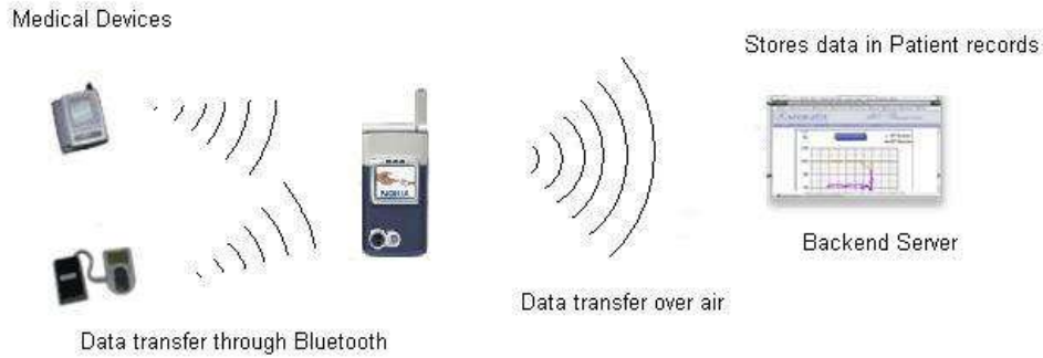
Fig 2: Mobile Monitoring (via Mobile Phone)
